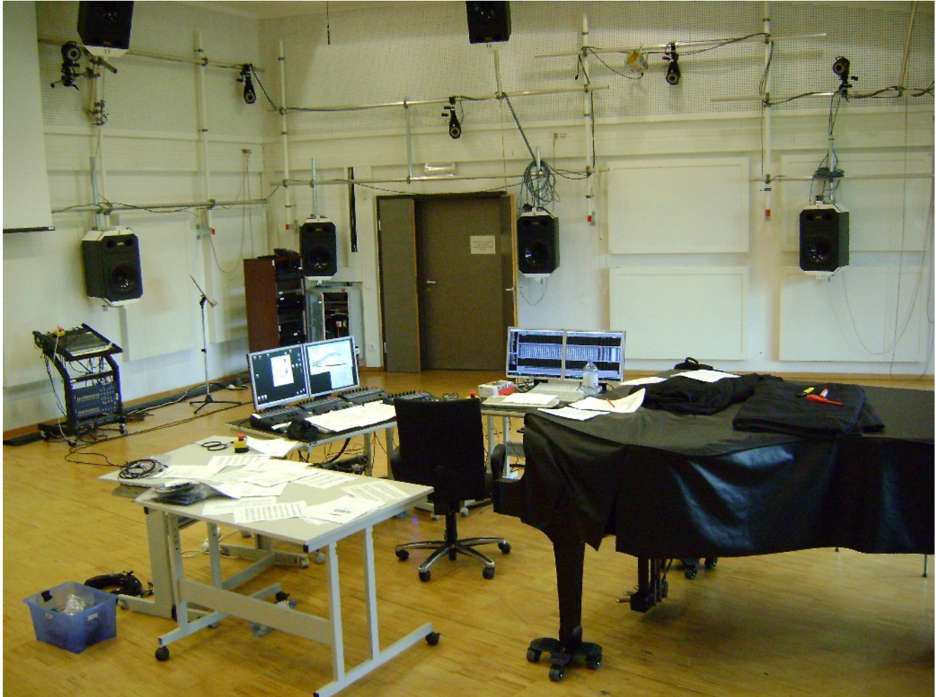
Illustration 3: Post-production at the IEM Cube in Graz, on a 24-speaker hemisphere of Tannoy 1200s. The console on the left controls the CUBEMixer. The MIDI controllers are attached to the machine on the right, which runs the Ardour session. The grand piano was extremely handy while working with the score. The two red buttons on the tables are emergency-mute switches for the speaker system.
